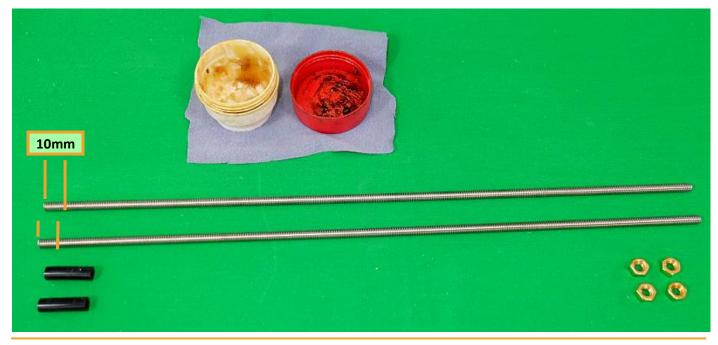
Grease the threaded rods and make the nuts circulate from one end to another in order to spread the grease.
