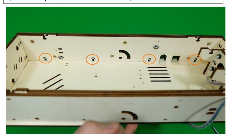
Tighten screws corresponding to the holes, head contact, loosely.
