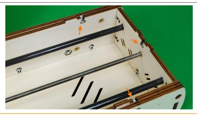
Gently put on the aluminum cover and loosely tighten the end screws M4x10.
