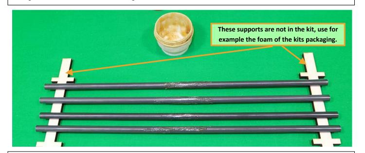
Spread the grease with a cloth, a thin film is sufficient.
