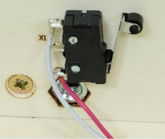
For **XC** <u>and</u> **XL**, place the screws <u>in the left position of the setting area</u> and tighten moderately, without marking the wood so as to be able to adjust the position later.
