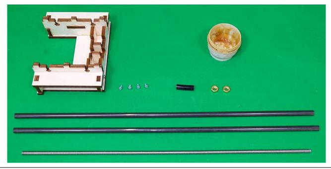
As with the threaded rods of the gantry, screw in the nuts on the side marked in blue or green and screw the sleeve on the opposite side 10mm. Lubricate the threaded rod, spread the grease with the nuts and remove the excess.
