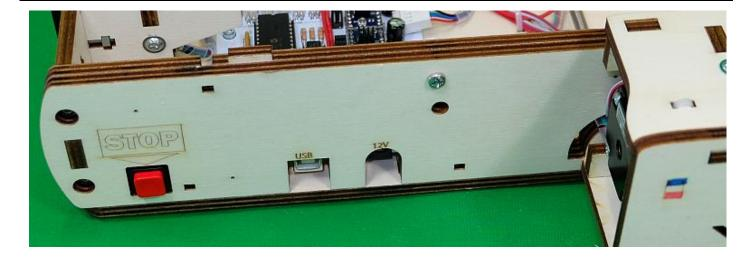
Loosen the black knobs and straighten the gantry. Check that the cables do follow the movement in the base. Perform several movements of folding-unfolding to check that all is going well and that the cables do not stick in the quarter circle holes.
