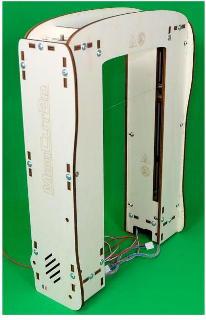
Lay down the gantry with the hand engraved facing up and slide it around the base of the MiniCut2d.
