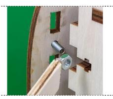
The engines on the MiniCut2d are mounted on silent-blocks (to reduce operating noise). The silent-blocks have a precise length, careful not to mix the different bags.
