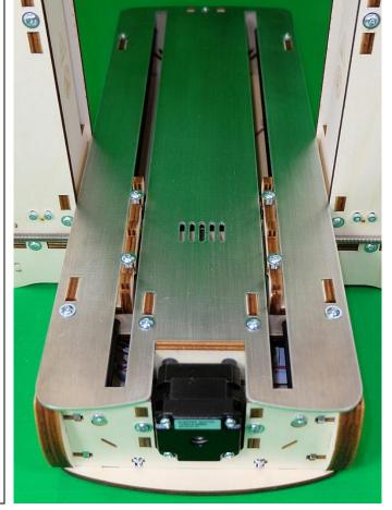
Unscrew the 4 screws M4x16 (without dropping the nuts).
