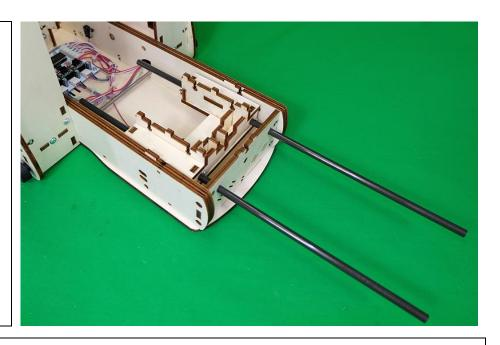
Push the bars fully in the plywood holes and secure them with 2.9x6.5mm screws on both sides.
